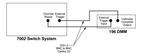
Figure 4-20 External trigger connectors
