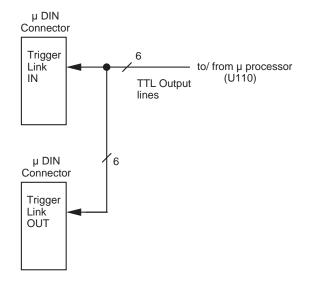
**Figure 6-9** Trigger link
