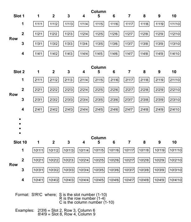
Figure 4-11 Channel assignments (matrix cards)
