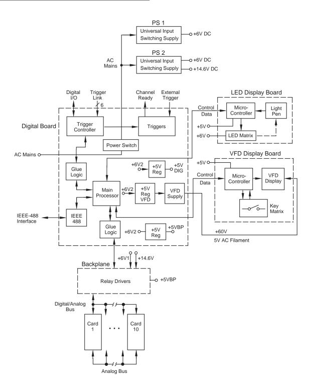
Figure 6-1 Model 7002 system block diagram
