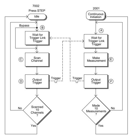
**Figure 4-24**Operation model for asynchronous Trigger Link example #1
