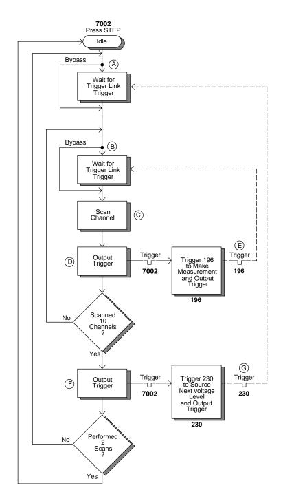
**Figure 4-28**Operation model for asynchronous Trigger Link example #2
